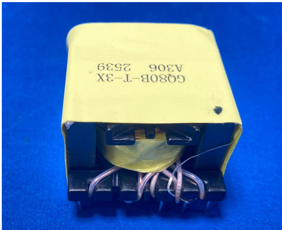
Photo -8 External view_3 of transformer T1
